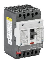
Gladiator molded case circuit breaker, 100A frame, 80A, 600Y / 480 VAC / 500 VDC, 3-pole, characteristics, fixed thermal/fixed magnetic, 35kA @ 480 VAC interrupting rating, panel mount. Line and load lug terminals included.
