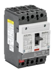
Gladiator molded case circuit breaker, 100A frame, 70A, 600Y / 480 VAC / 500 VDC, 3-pole, characteristics, fixed thermal/fixed magnetic, 35kA @ 480 VAC interrupting rating, panel mount. Line and load lug terminals included.
