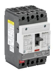
Gladiator molded case circuit breaker, 100A frame, 60A, 600Y / 480 VAC / 500 VDC, 3-pole, characteristics, fixed thermal/fixed magnetic, 35kA @ 480 VAC interrupting rating, panel mount. Line and load lug terminals included.
