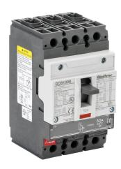
Gladiator molded case circuit breaker, 100A frame, 50A, 600Y / 480 VAC / 500 VDC, 3-pole, characteristics, fixed thermal/fixed magnetic, 35kA @ 480 VAC interrupting rating, panel mount. Line and load lug terminals included.
