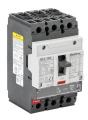
Gladiator molded case circuit breaker, 100A frame, 50A, 600Y / 480 VAC / 500 VDC, 3-pole, characteristics, fixed thermal/fixed magnetic, 35kA @ 480 VAC interrupting rating, panel mount. Line and load lug terminals included.
