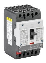
Gladiator molded case circuit breaker, 100A frame, 40A, 600Y / 480 VAC / 500 VDC, 3-pole, characteristics, fixed thermal/fixed magnetic, 35kA @ 480 VAC interrupting rating, panel mount. Line and load lug terminals included.
