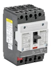
Gladiator molded case circuit breaker, 100A frame, 30A, 600Y / 480 VAC / 500 VDC, 3-pole, characteristics, fixed thermal/fixed magnetic, 35kA @ 480 VAC interrupting rating, panel mount. Line and load lug terminals included.
