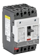
Gladiator molded case circuit breaker, 100A frame, 25A, 600Y / 480 VAC / 500 VDC, 3-pole, characteristics, fixed thermal/fixed magnetic, 35kA @ 480 VAC interrupting rating, panel mount. Line and load lug terminals included.
