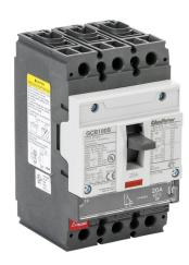
Gladiator molded case circuit breaker, 100A frame, 20A, 600Y / 480 VAC / 500 VDC, 3-pole, characteristics, fixed thermal/fixed magnetic, 35kA @ 480 VAC interrupting rating, panel mount. Line and load lug terminals included.
