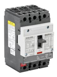
Gladiator molded case circuit breaker, 100A frame, 15A, 600Y / 480 VAC / 500 VDC, 3-pole, characteristics, fixed thermal/fixed magnetic, 35kA @ 480 VAC interrupting rating, panel mount. Line and load lug terminals included.
