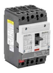
Gladiator molded case circuit breaker, 100A frame, 100A, 600Y / 480 VAC / 500 VDC, 3-pole, characteristics, fixed thermal/fixed magnetic, 35kA @ 480 VAC interrupting rating, panel mount. Line and load lug terminals included.
