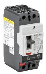
Gladiator molded case circuit breaker, 100A frame, 90A, 600Y / 480 VAC / 250 VDC, 2-pole, characteristics, fixed thermal/fixed magnetic, 35kA @ 480 VAC interrupting rating, panel mount. Line and load lug terminals included.
