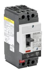
Gladiator molded case circuit breaker, 100A frame, 80A, 600Y / 480 VAC / 250 VDC, 2-pole, characteristics, fixed thermal/fixed magnetic, 35kA @ 480 VAC interrupting rating, panel mount. Line and load lug terminals included.
