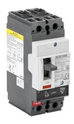
Gladiator molded case circuit breaker, 100A frame, 70A, 600Y / 480 VAC / 250 VDC, 2-pole, characteristics, fixed thermal/fixed magnetic, 35kA @ 480 VAC interrupting rating, panel mount. Line and load lug terminals included.
