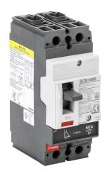
Gladiator molded case circuit breaker, 100A frame, 60A, 600Y / 480 VAC / 250 VDC, 2-pole, characteristics, fixed thermal/fixed magnetic, 35kA @ 480 VAC interrupting rating, panel mount. Line and load lug terminals included.
