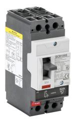
Gladiator molded case circuit breaker, 100A frame, 50A, 600Y / 480 VAC / 250 VDC, 2-pole, characteristics, fixed thermal/fixed magnetic, 35kA @ 480 VAC interrupting rating, panel mount. Line and load lug terminals included.
