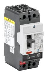
Gladiator molded case circuit breaker, 100A frame, 40A, 600Y / 480 VAC / 250 VDC, 2-pole, characteristics, fixed thermal/fixed magnetic, 35kA @ 480 VAC interrupting rating, panel mount. Line and load lug terminals included.
