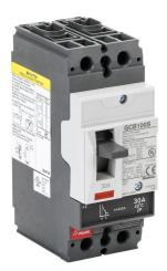
Gladiator molded case circuit breaker, 100A frame, 30A, 600Y / 480 VAC / 250 VDC, 2-pole, characteristics, fixed thermal/fixed magnetic, 35kA @ 480 VAC interrupting rating, panel mount. Line and load lug terminals included.
