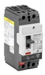
Gladiator molded case circuit breaker, 100A frame, 20A, 600Y / 480 VAC / 250 VDC, 2-pole, characteristics, fixed thermal/fixed magnetic, 35kA @ 480 VAC interrupting rating, panel mount. Line and load lug terminals included.
