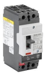
Gladiator molded case circuit breaker, 100A frame, 15A, 600Y / 480 VAC / 250 VDC, 2-pole, characteristics, fixed thermal/fixed magnetic, 35kA @ 480 VAC interrupting rating, panel mount. Line and load lug terminals included.
