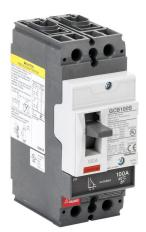
Gladiator molded case circuit breaker, 100A frame, 100A, 600Y / 480 VAC / 250 VDC, 2-pole, characteristics, fixed thermal/fixed magnetic, 35kA @ 480 VAC interrupting rating, panel mount. Line and load lug terminals included.
