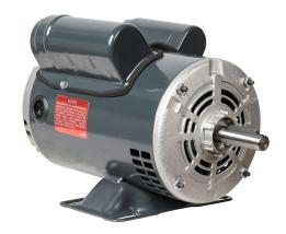
Marathon standard efficiency AC induction motor, general purpose, 3/4hp, 1-phase, 115/230 VAC, suitable for 208 VAC at 60 Hz, 3600rpm, ODP, NEMA 56 frame, rolled steel, rigid base mount.
