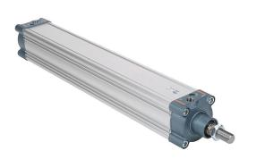
NITRA pneumatic cylinder, ISO 15552, 80mm bore, 25mm rod diameter, 500mm stroke, double acting, magnetic piston, front and rear adjustable cushions.
