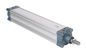
NITRA pneumatic cylinder, ISO 15552, 80mm bore, 25mm rod diameter, 400mm stroke, double acting, magnetic piston, front and rear adjustable cushions.
