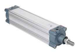
NITRA pneumatic cylinder, ISO 15552, 80mm bore, 25mm rod diameter, 300mm stroke, double acting, magnetic piston, front and rear adjustable cushions.
