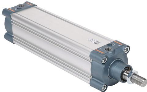
NITRA pneumatic cylinder, ISO 15552, 80mm bore, 25mm rod diameter, 250mm stroke, double acting, magnetic piston, front and rear adjustable cushions.
