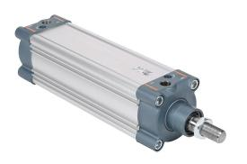
NITRA pneumatic cylinder, ISO 15552, 80mm bore, 25mm rod diameter, 200mm stroke, double acting, magnetic piston, front and rear adjustable cushions.
