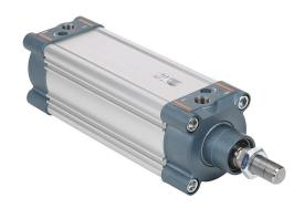
NITRA pneumatic cylinder, ISO 15552, 80mm bore, 25mm rod diameter, 150mm stroke, double acting, magnetic piston, front and rear adjustable cushions.
