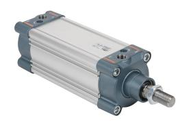
NITRA pneumatic cylinder, ISO 15552, 80mm bore, 25mm rod diameter, 125mm stroke, double acting, magnetic piston, front and rear adjustable cushions.
