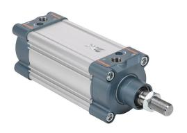
NITRA pneumatic cylinder, ISO 15552, 80mm bore, 25mm rod diameter, 100mm stroke, double acting, magnetic piston, front and rear adjustable cushions.
