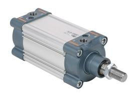
NITRA pneumatic cylinder, ISO 15552, 80mm bore, 25mm rod diameter, 75mm stroke, double acting, magnetic piston, front and rear adjustable cushions.
