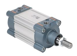
NITRA pneumatic cylinder, ISO 15552, 80mm bore, 25mm rod diameter, 50mm stroke, double acting, magnetic piston, front and rear adjustable cushions.
