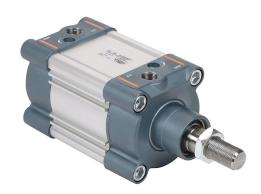
NITRA pneumatic cylinder, ISO 15552, 80mm bore, 25mm rod diameter, 25mm stroke, double acting, magnetic piston, front and rear adjustable cushions.
