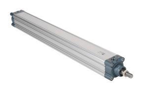
NITRA pneumatic cylinder, ISO 15552, 63mm bore, 20mm rod diameter, 600mm stroke, double acting, magnetic piston, front and rear adjustable cushions.
