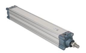
NITRA pneumatic cylinder, ISO 15552, 63mm bore, 20mm rod diameter, 400mm stroke, double acting, magnetic piston, front and rear adjustable cushions.
