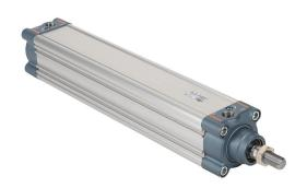
NITRA pneumatic cylinder, ISO 15552, 63mm bore, 20mm rod diameter, 300mm stroke, double acting, magnetic piston, front and rear adjustable cushions.
