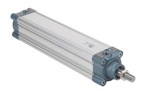
NITRA pneumatic cylinder, ISO 15552, 63mm bore, 20mm rod diameter, 250mm stroke, double acting, magnetic piston, front and rear adjustable cushions.
