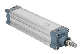
NITRA pneumatic cylinder, ISO 15552, 63mm bore, 20mm rod diameter, 200mm stroke, double acting, magnetic piston, front and rear adjustable cushions.
