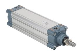
NITRA pneumatic cylinder, ISO 15552, 63mm bore, 20mm rod diameter, 150mm stroke, double acting, magnetic piston, front and rear adjustable cushions.
