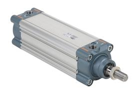
NITRA pneumatic cylinder, ISO 15552, 63mm bore, 20mm rod diameter, 125mm stroke, double acting, magnetic piston, front and rear adjustable cushions.
