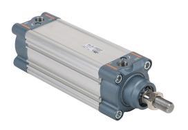
NITRA pneumatic cylinder, ISO 15552, 63mm bore, 20mm rod diameter, 100mm stroke, double acting, magnetic piston, front and rear adjustable cushions.
