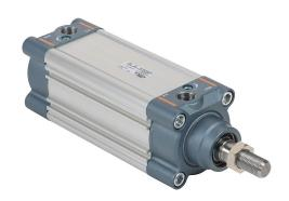
NITRA pneumatic cylinder, ISO 15552, 63mm bore, 20mm rod diameter, 75mm stroke, double acting, magnetic piston, front and rear adjustable cushions.
