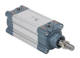
NITRA pneumatic cylinder, ISO 15552, 63mm bore, 20mm rod diameter, 50mm stroke, double acting, magnetic piston, front and rear adjustable cushions.
