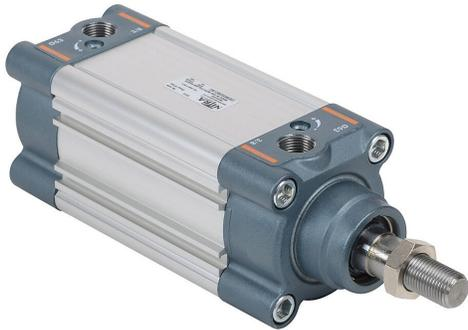
NITRA pneumatic cylinder, ISO 15552, 63mm bore, 20mm rod diameter, 50mm stroke, double acting, magnetic piston, front and rear adjustable cushions.
