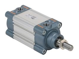
NITRA pneumatic cylinder, ISO 15552, 63mm bore, 20mm rod diameter, 25mm stroke, double acting, magnetic piston, front and rear adjustable cushions.
