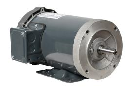
Marathon XRI premium efficiency AC induction motor, general purpose, inverter rated and 4-in-1, 1-1/2hp, 3-phase, 230/460 VAC, suitable for 208 VAC at 60 Hz, 1800rpm, TEFC, NEMA 56HC frame, rolled steel, C-face/removable rigid base mount.
