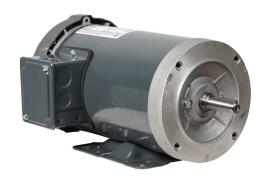
Marathon XRI premium efficiency AC induction motor, general purpose, inverter rated and 4-in-1, 1-1/2hp, 3-phase, 230/460 VAC, suitable for 208 VAC at 60 Hz, 1800rpm, TEFC, 56HC frame, rolled steel, C-face/removable rigid base mount.
