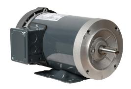
Marathon XRI premium efficiency AC induction motor, general purpose, inverter rated and 4-in-1, 1hp, 3-phase, 230/460 VAC, suitable for 208 VAC at 60 Hz, 1800rpm, TEFC, 56HC frame, rolled steel, C-face/removable rigid base mount.
