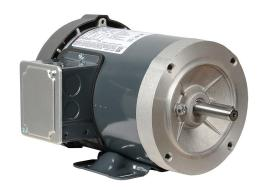
Marathon XRI standard efficiency AC induction motor, general purpose, inverter rated and 4-in-1, 3/4hp, 3-phase, 208-230/460 VAC, 1800rpm, TEFC, NEMA 56C frame, rolled steel, C-face/removable rigid base mount.
