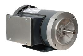
Marathon standard efficiency AC induction motor, general purpose and 4-in-1, 1-1/2hp, 1-phase, 115/208-230 VAC, 1800rpm, TEFC, NEMA 56HC frame, rolled steel, C-face/removable rigid base mount.
