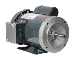
Marathon standard efficiency AC induction motor, general purpose and 4-in-1, 1hp, 1-phase, 115/208-230 VAC, 1800rpm, TEFC, NEMA 56HC frame, rolled steel, C-face/removable rigid base mount.
