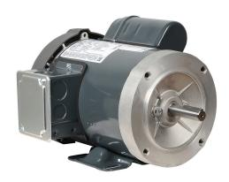
Marathon standard efficiency AC induction motor, general purpose and 4-in-1, 3/4hp, 1-phase, 115/208-230 VAC, 1800rpm, TEFC, NEMA 56C frame, rolled steel, C-face/removable rigid base mount.
