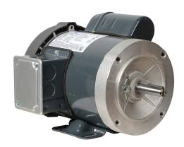
Marathon standard efficiency AC induction motor, general purpose and 4-in-1, 1/3hp, 1-phase, 115/208-230 VAC, 1800rpm, TEFC, 56C frame, rolled steel, C-face/removable rigid base mount.
